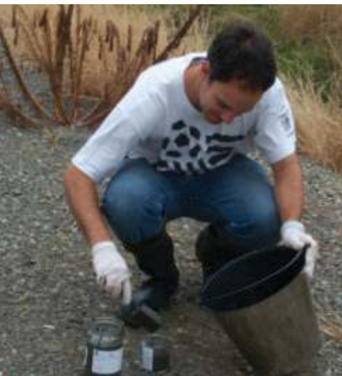
Transferring sediment into jars to be shipped to the analytical laboratories. Photo courtesy of Paul Salop.
